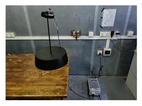
Radiated Emissions, 30MHz to 1GHz Test Setup
