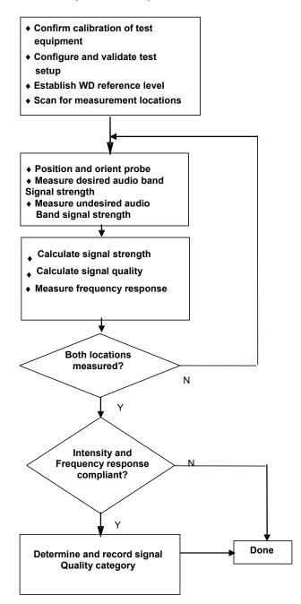
Figure 4-15 C63.19 T-Coil Signal Test Process
