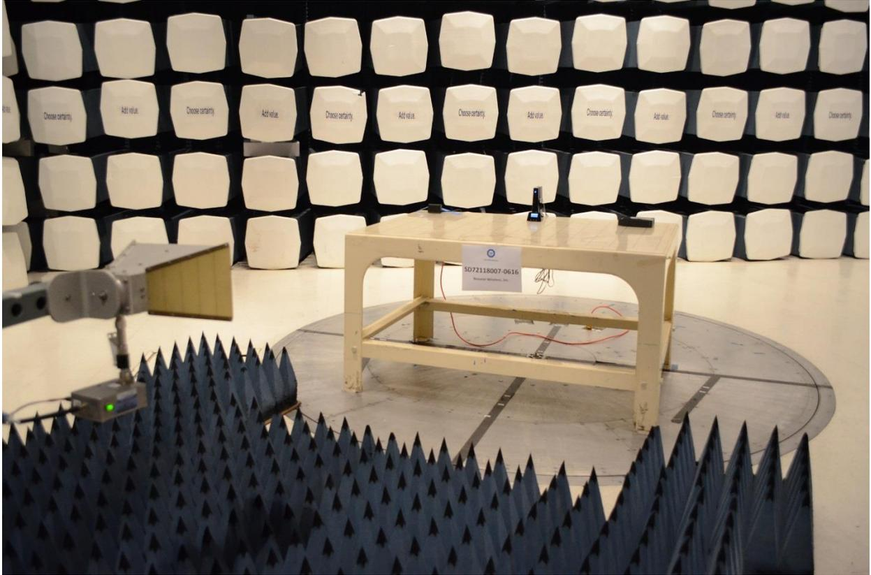
**Radiated Emissions Test Setup (above 1GHz Front)**
