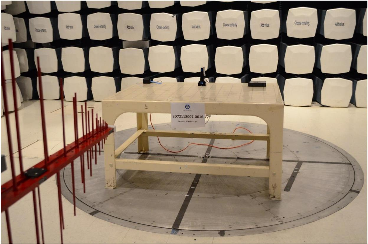
**Radiated Emissions Test Setup (below 1GHz Front)**
