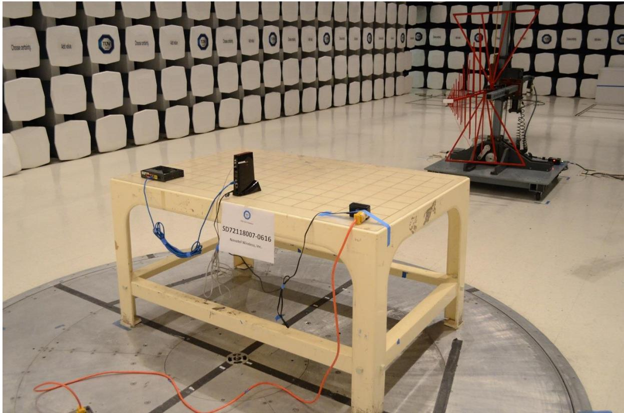
**Radiated Emissions Test Setup (below 1GHz Back)**
