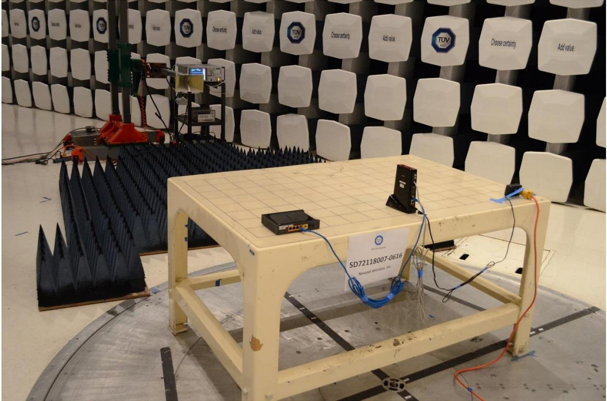
**Radiated Emissions Test Setup (above 1GHz Back)**
