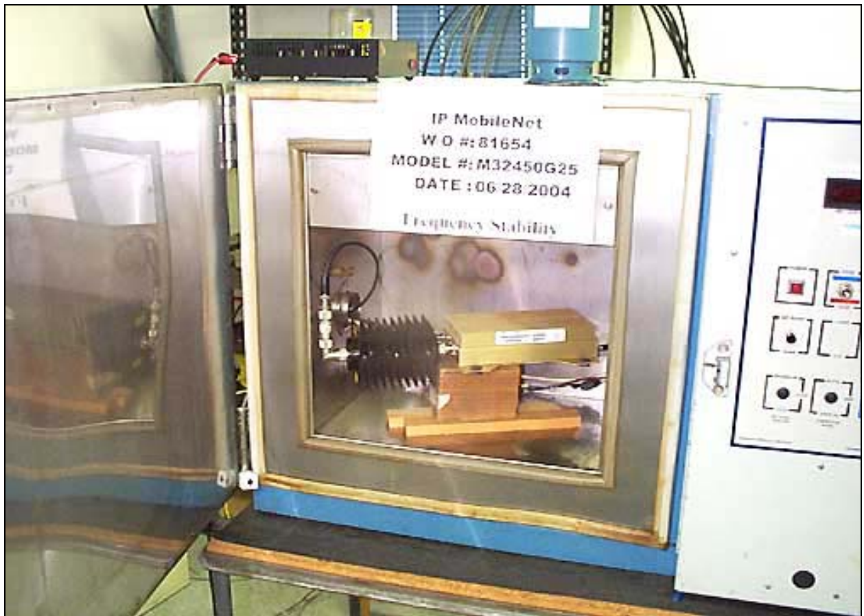
PHOTOGRAPH SHOWING TEMPERATURE TESTING
