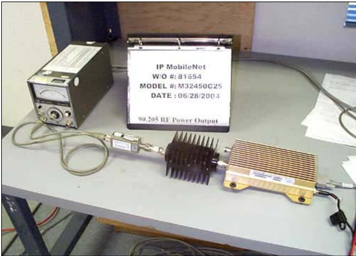
PHOTOGRAPH SHOWING RF POWER OUTPUT
