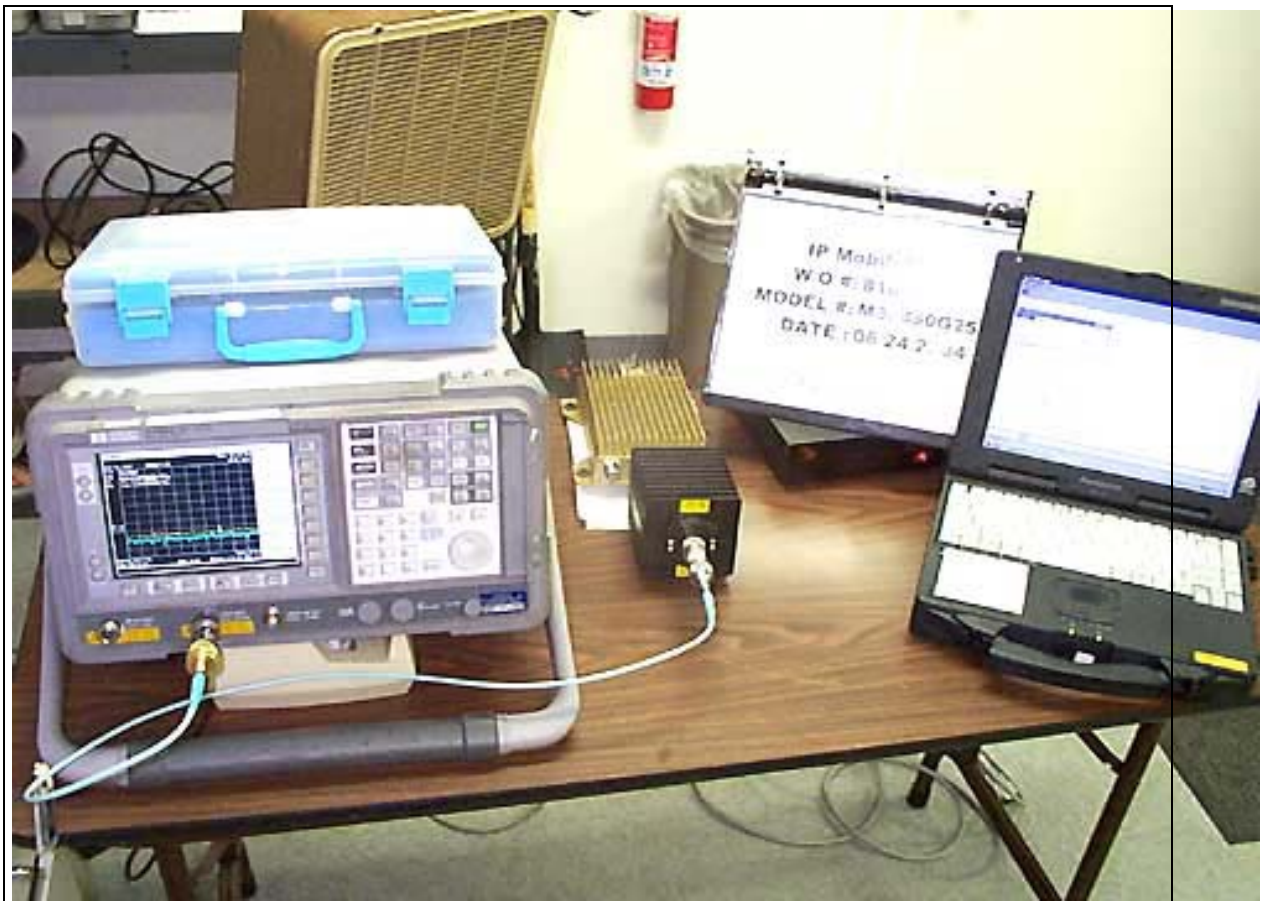
PHOTOGRAPH SHOWING DIRECT CONNECT TEST SETUP
