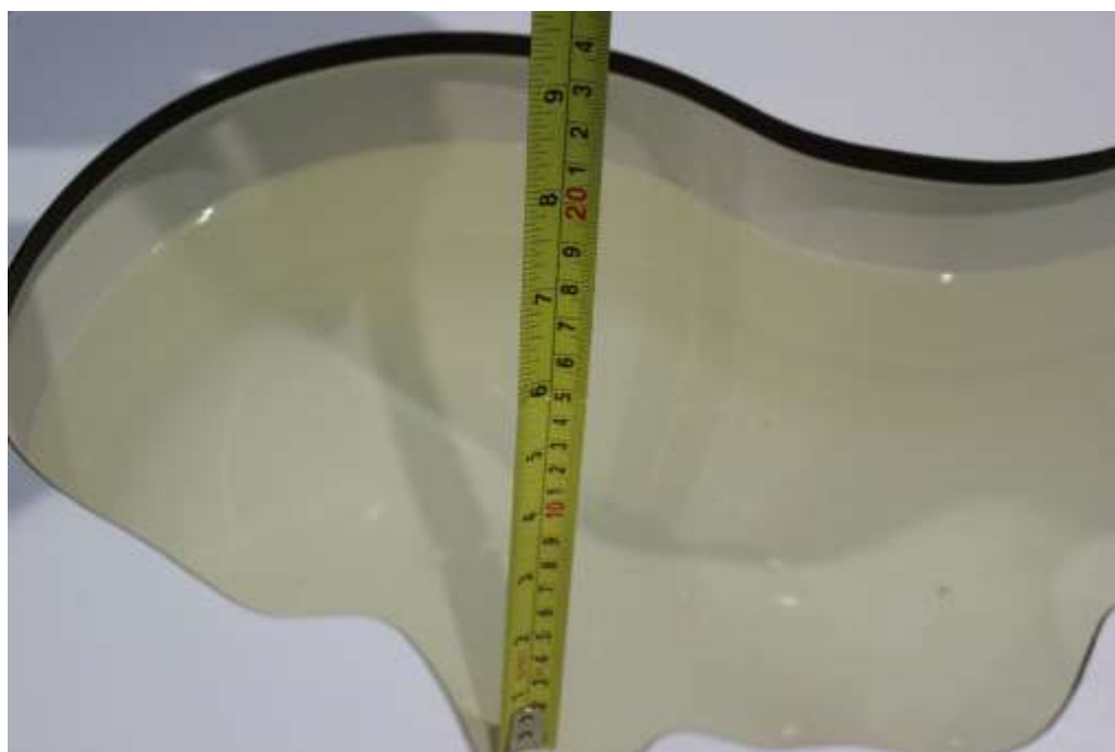
Picture 7-7: Liquid depth in the Head Phantom(5GHz)
