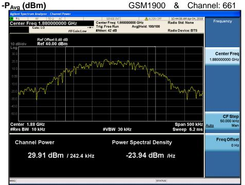
$PAPR (dB) = P_{Pk} (dBm) - P_{Avg} (dBm) = 30.35 dBm - 29.91 dBm = 0.44 dB$
