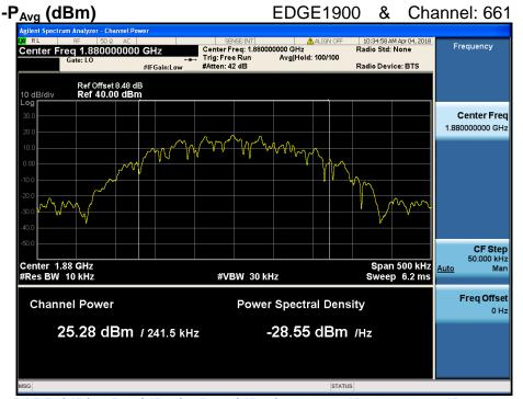
$PAPR(dB) = P_{Pk}(dBm) - P_{Avg}(dBm) = 28.96 dBm - 25.28 dBm = 3.68 dB$
