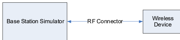
Figure 9-2 Power Measurement Setup
