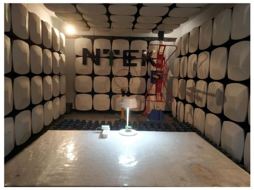
RADIATED EMISSION TEST SETUP 30M-1GHz
