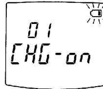
Switching the battery charging "01" On.
