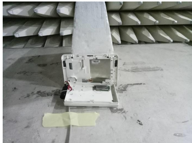
Photograph 8.1.2 Setup for radiated emission measurements, EUT cabling
