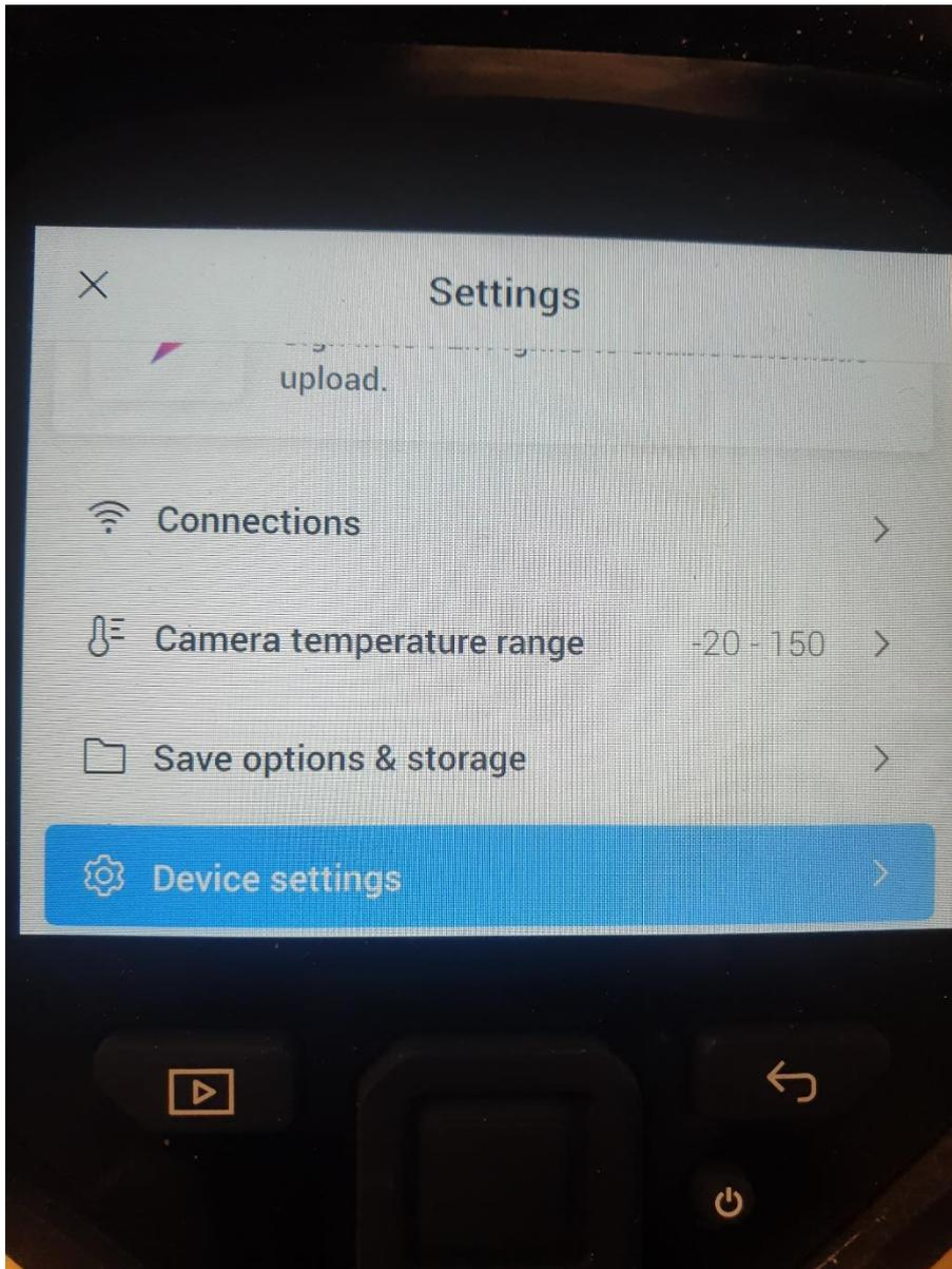
Figure 3 Press Device Settings
