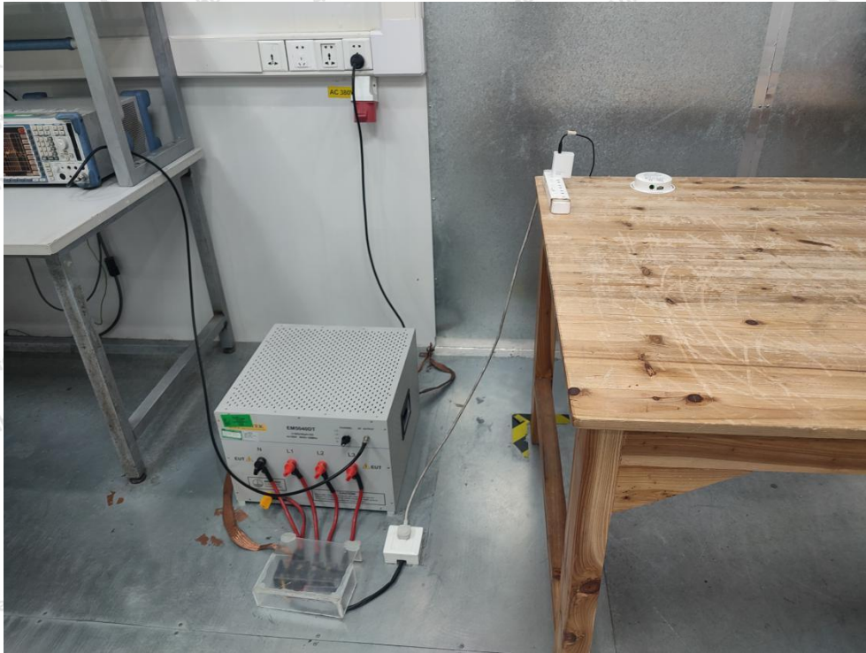
Photo of Conducted Emission Measurement
