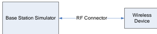
Figure 9-3 Power Measurement Setup
