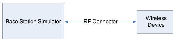
Figure 9-2 Power Measurement Setup
