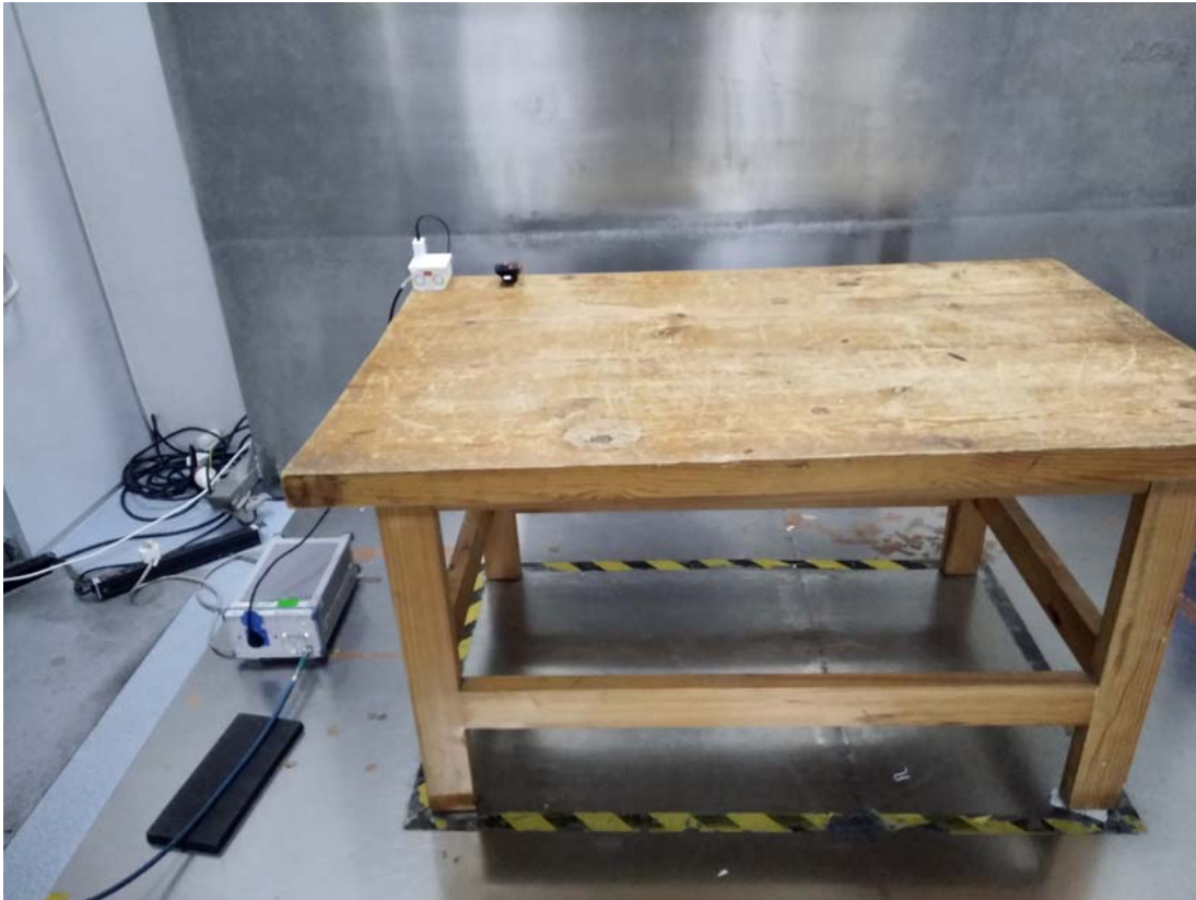
Conducted Emissions Side View
