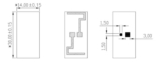
Figure 1 Physical dimension (mm)
