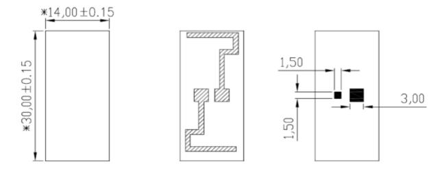
Figure 1 Physical dimension (mm)
