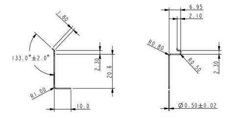
Figure 1 Physical dimension (mm)
