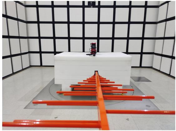
Radiated Emission 30 MHz-1 GHz View Front DC output + rear DC input + USB2.0 Link to Laptop
