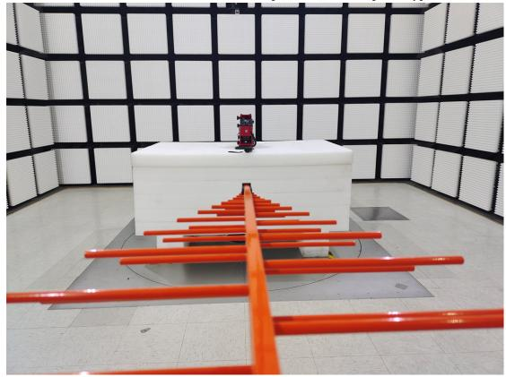
Radiated Emission 9 kHz-30 MHz Parallel ViewFront DC input + rear DC output + Type-C Link to Laptop
