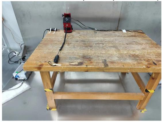
Conducted Emissions Side View Front DC output + rear DC input + USB2.0 Link to Laptop
