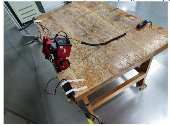
Conducted Emissions Front View Front DC output + rear DC input + Type-C Link to Laptop
