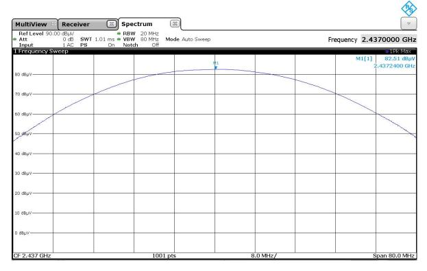
The antenna gain is below 6 dBi, therefore no conducted output limit reduction is necessary.
