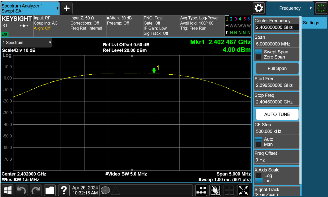
Figure 4: Peak Output Power, 2402MHz, BLE-2Mbps
