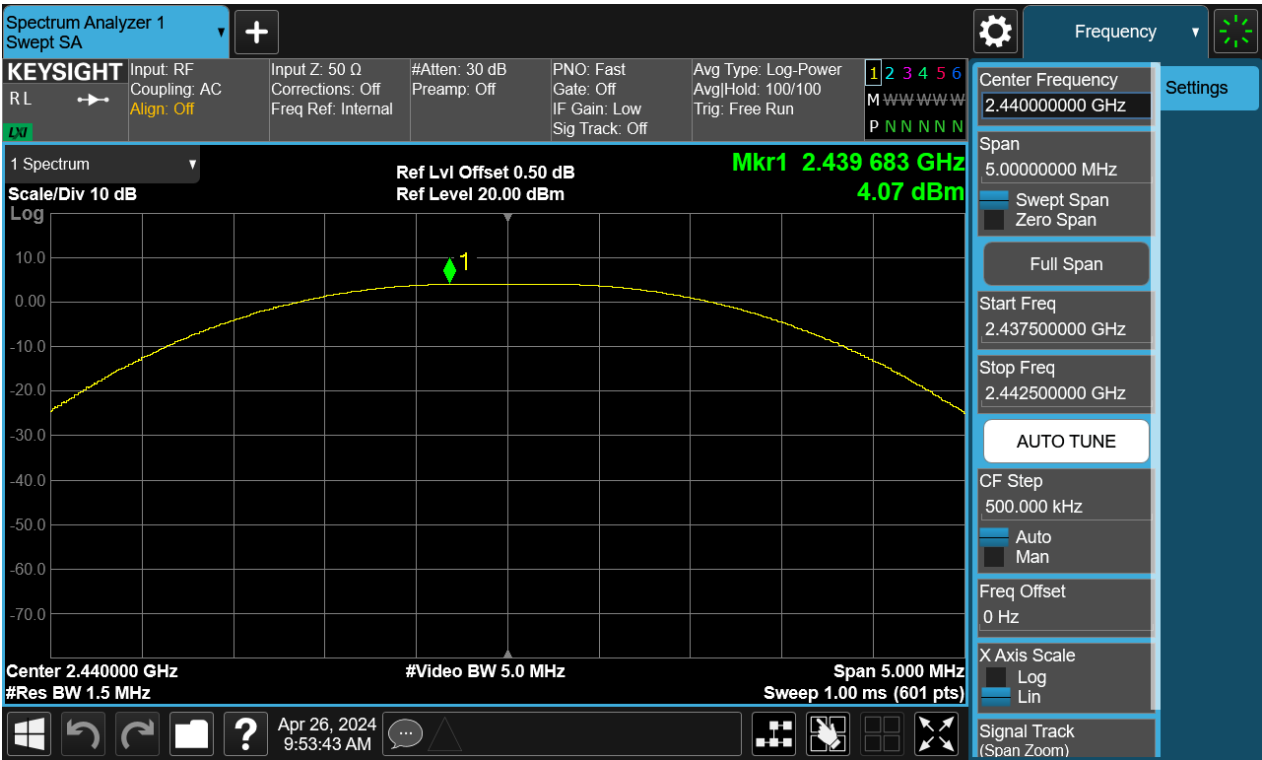
Figure 2: Peak Output Power, 2440MHz, BLE-1Mbps
