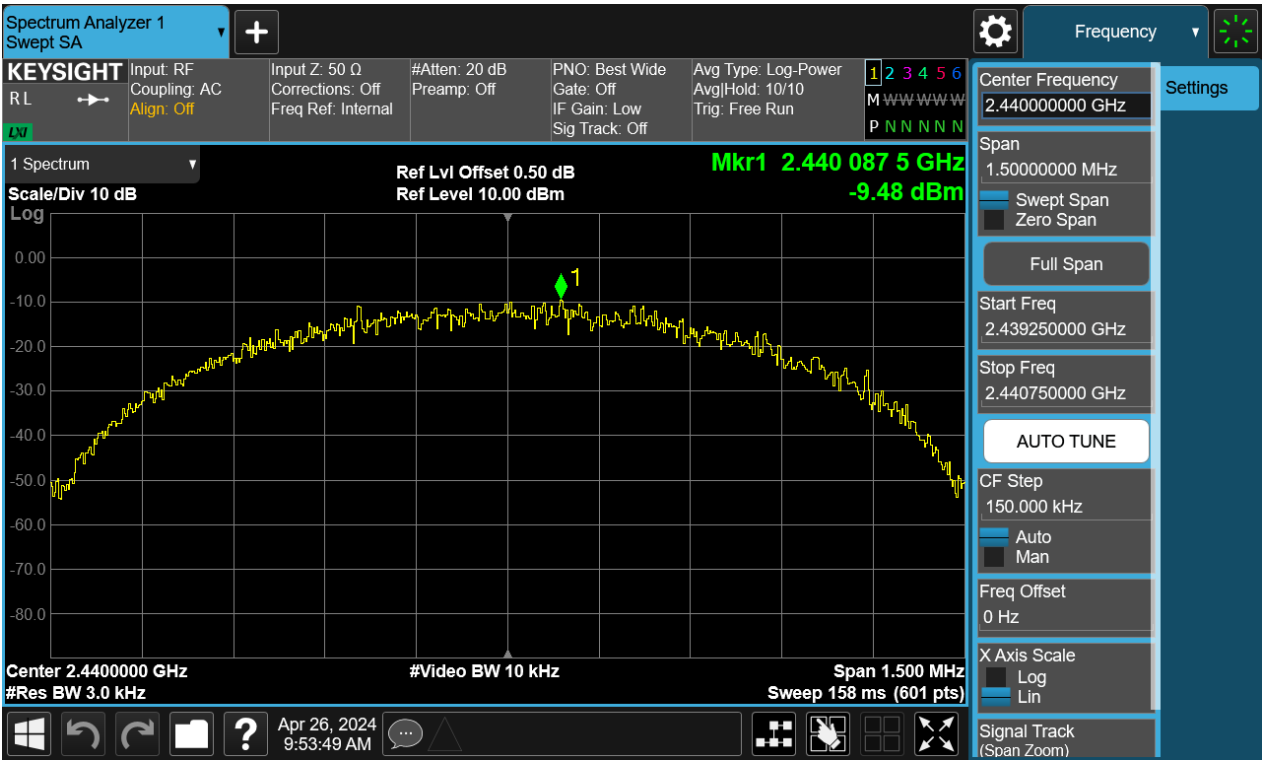
Figure 14: Power Spectral Density, 2440MHz, BLE-1Mbps
