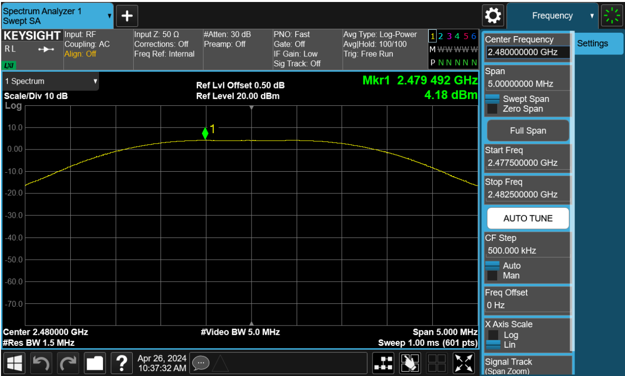
Figure 6: Peak Output Power, 2480MHz, BLE-2Mbps
