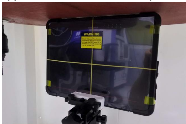
Edge 1 of EUT with Phantom 0 mm Gap
