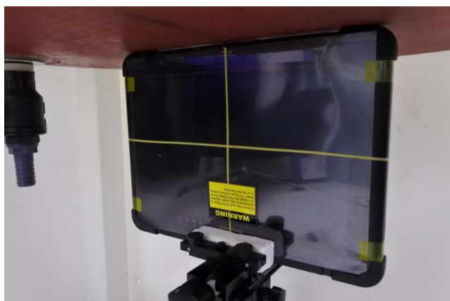
Edge 3 of EUT with Phantom 0 mm Gap
