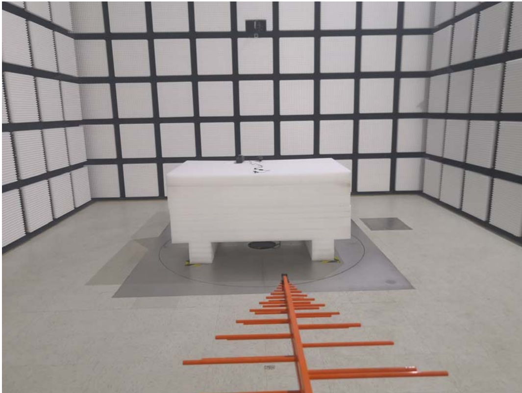
Radiated Emissions Below 1G Rear View-TM1
