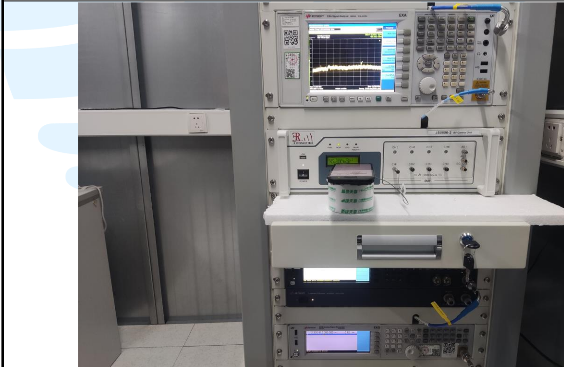
RF Conducted Test Setup
