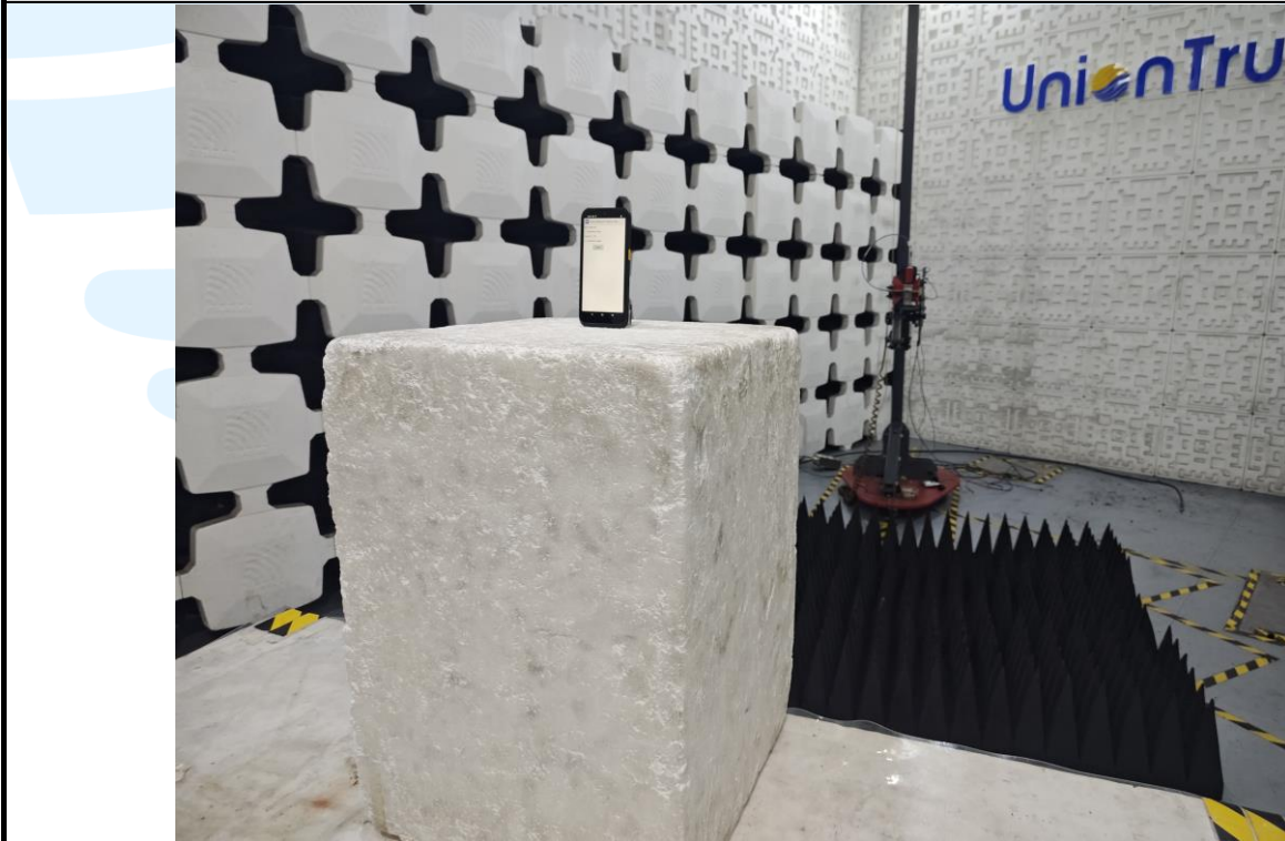
Radiated emission Test Setup (Above 1 GHz)
