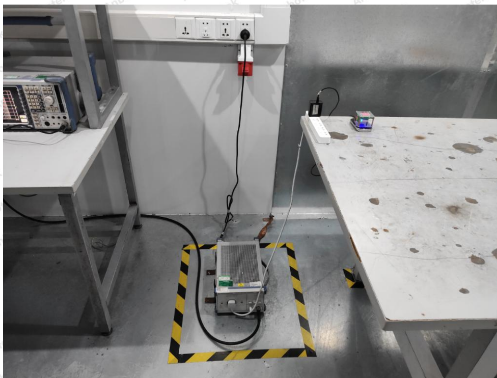
Photo of Conducted Emission Measurement
