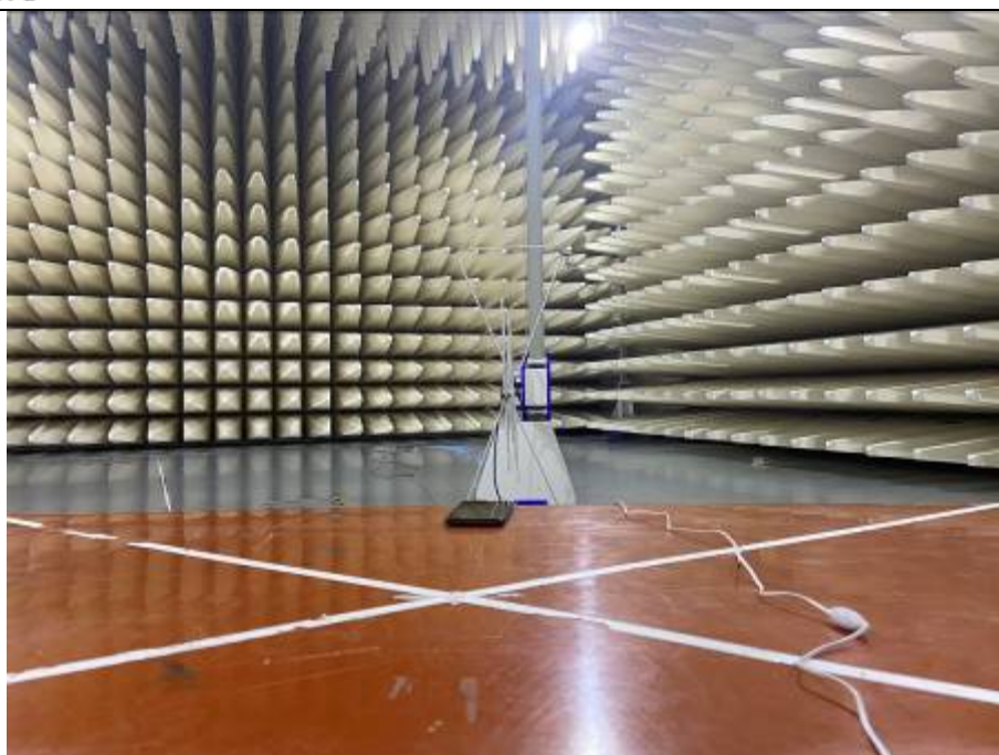
Radiated Emissions Test Setup (with charger) (30-1000MHz)
