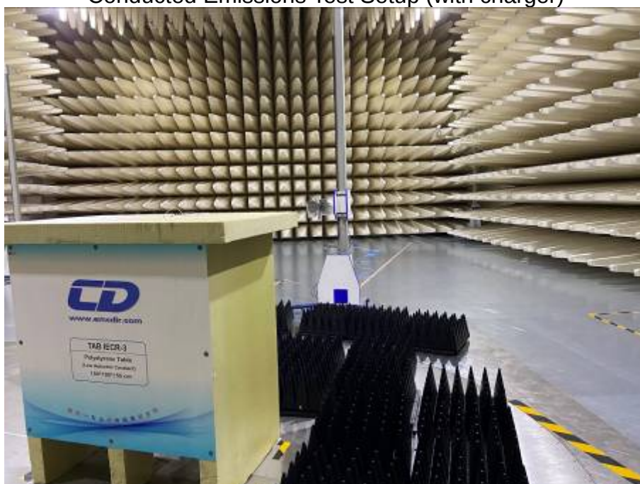
Conducted Emissions Test Setup (with charger)
