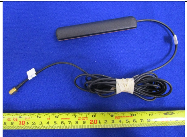
LTE/WCDMA Antenna – Top View
