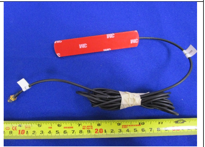
LTE/WCDMA Antenna – Bottom Side
