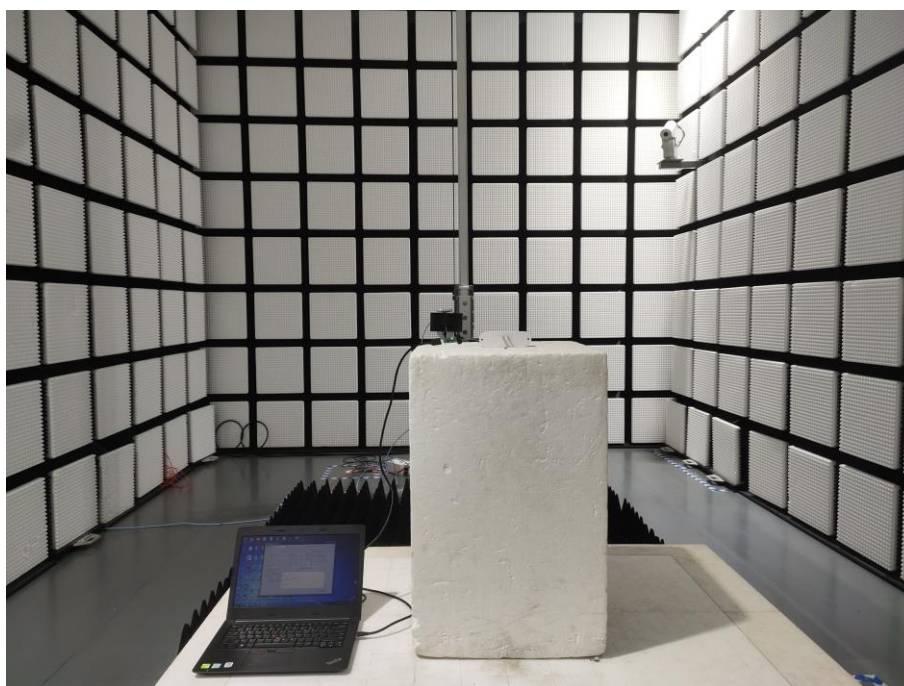
Fig. 3 Radiated emission setup photo(Above 1GHz)
