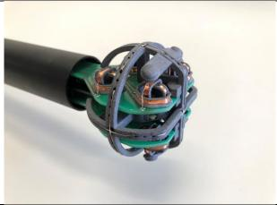
Test probe, without the casing
