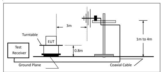
(c) For radiated emissions above 1000MHz
