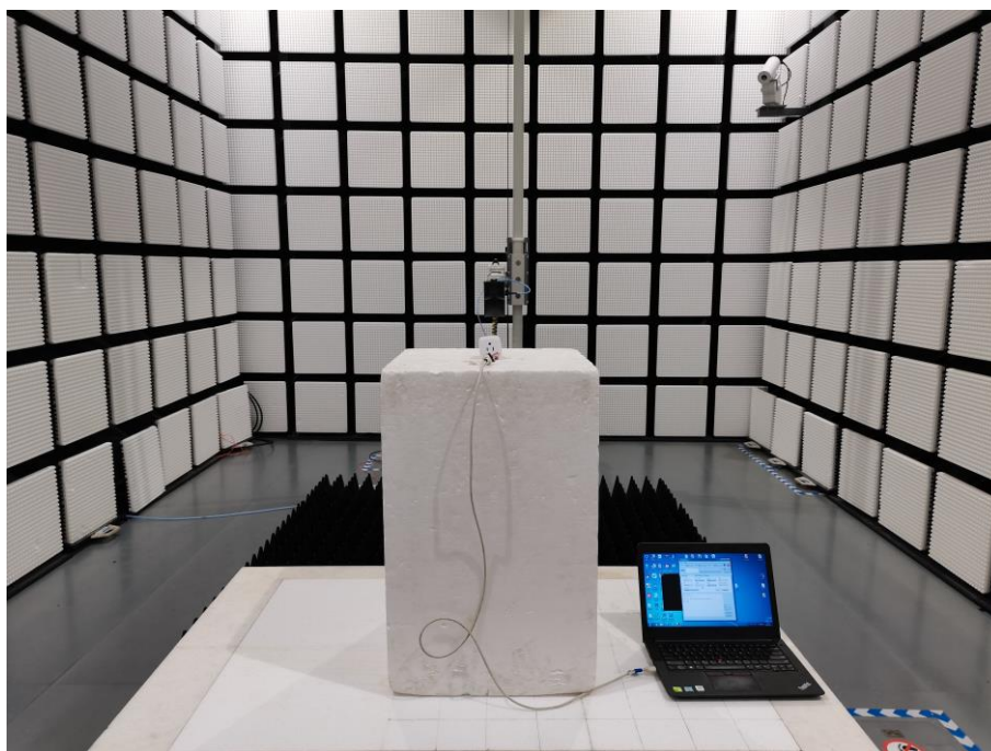
Fig. 3 Radiated emission setup photo(Above 1GHz)
