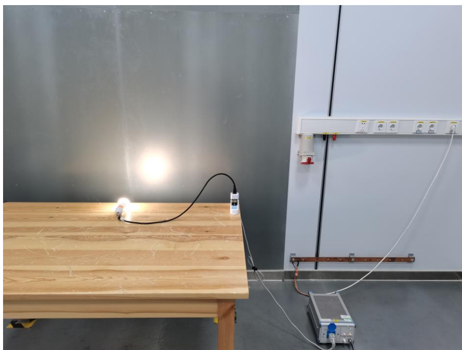
Fig. 4 Power line conducted emission setup photo
