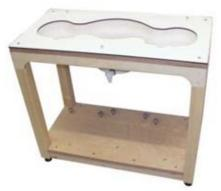
the phantom allow the complete set-up of all predefined phantom positions and measurement grids by manually teaching three points in the robot.
