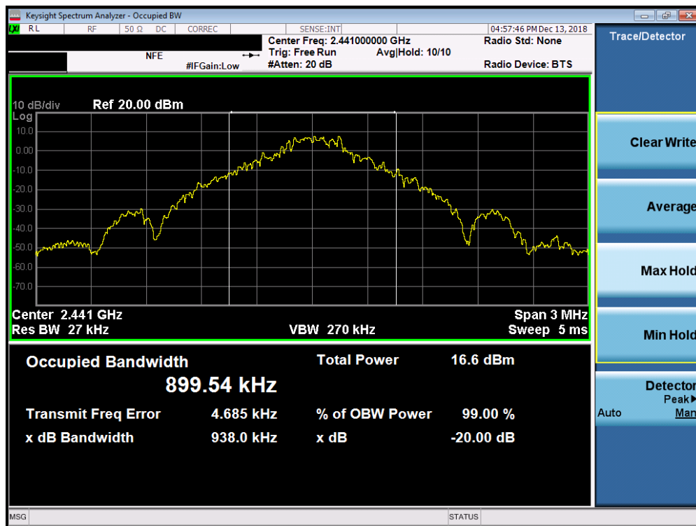
Plot 7-2. 20dB Bandwidth Plot (Bluetooth, 1Mbps – Ch. 39)
