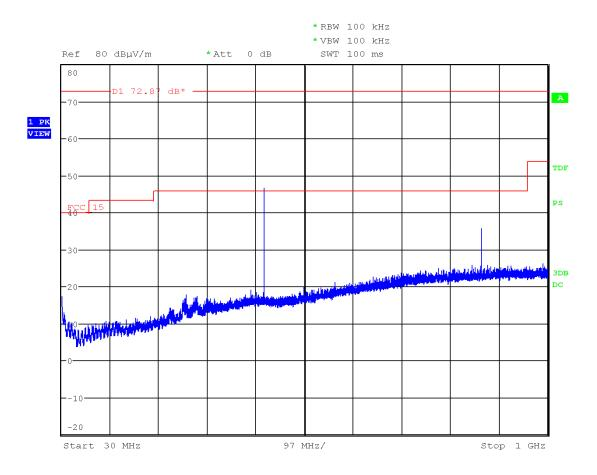
Note: For spurious emissions measurement the carrier frequency (fundamental) was attenuated using a notch filter.
