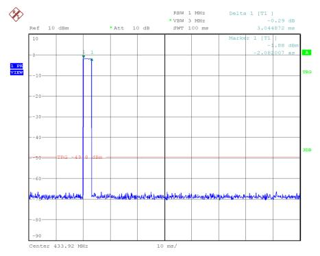
The equipment transmits one pulse of 3.04 ms every 19.90 seconds (see plots above). 30 times the duration of the transmission is 91.20 miliseconds.
