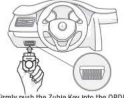
Firmly push the Zubie Key into the OBDII port (underneath your dashboard).
