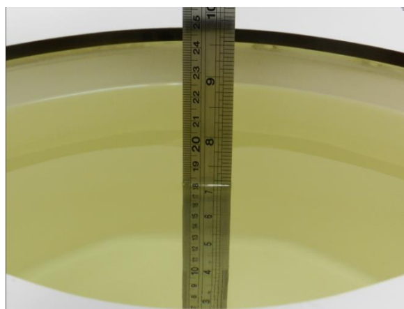
Fig 10.2 Photo of Liquid Height for Body SAR
