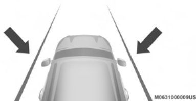
Lane Sensed (Solid Yellow Inside Line, Solid Yellow Outside Line) With Solid Yellow Telltale
