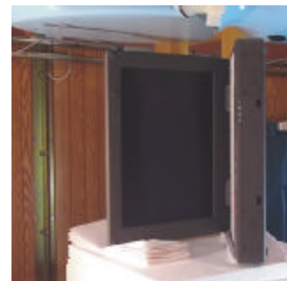
Body SAR Test Setup with 2.0cm separation distance
