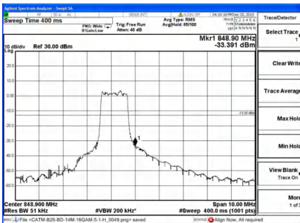
Band26-High Channel-3MHz Bandwidth-6RB-QPSK
