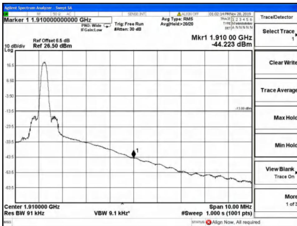
Band2-High Channel-5MHz Bandwidth-1RB-QPSK
