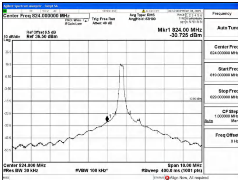
Band26-Low Channel-10MHz Bandwidth-1RB-16QAM
