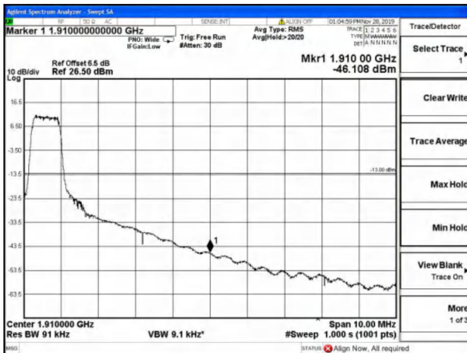
Band2-High Channel-5MHz Bandwidth-6RB-16QAM
