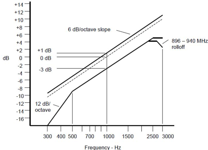
An additional 6 dB per octave attenuation is allowed from 2500 Hz to 3000 Hz in equipment operating in the 25 MHz to 869 MHz range.
