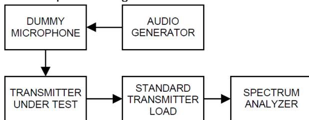
Test setup for Digital:
