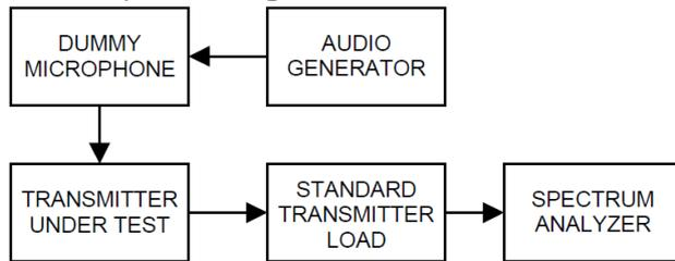
Test setup for Digital:
