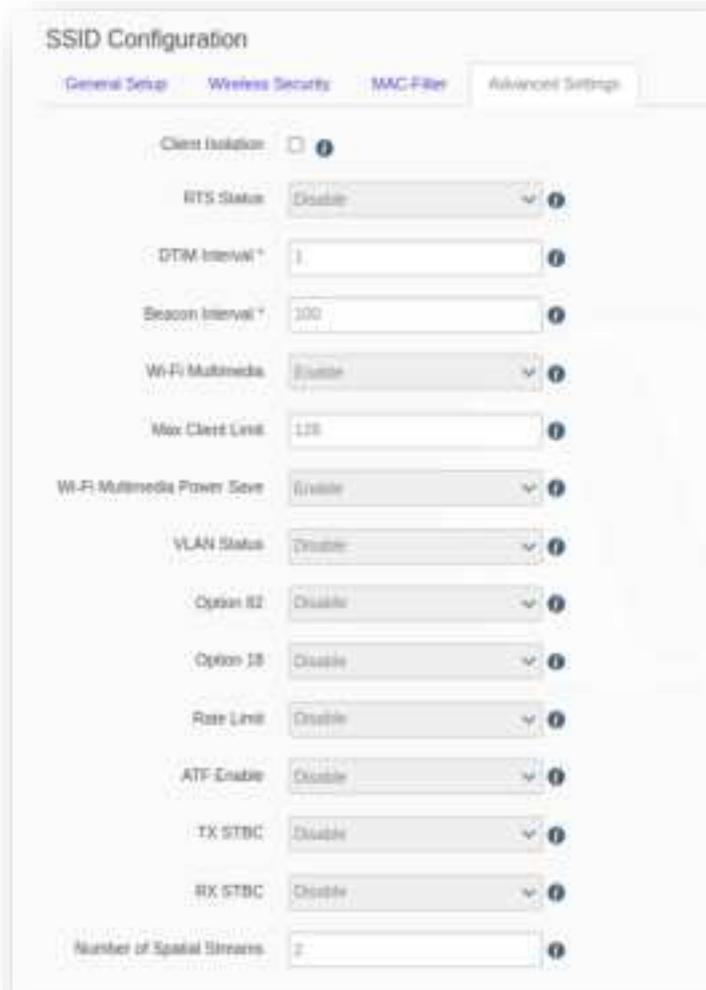
Figure 29: SSID Configuration Advanced Setting
