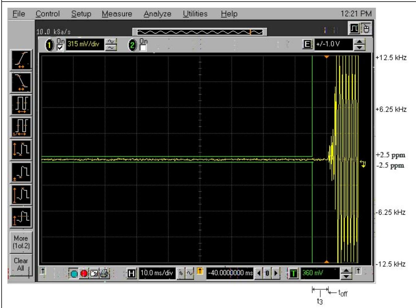
**Plot 5.12.3.3. Transient Frequency Behavior for 25 kHz Channel Spacing**
