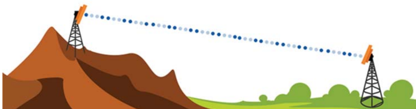
Figure 8-2 Typical installation showing device/antenna tilt angle
