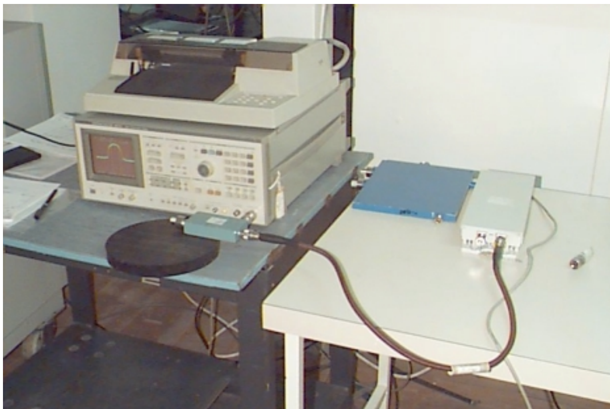
Photograph 1.1.1 Setup for minimum bandwidth measurements
