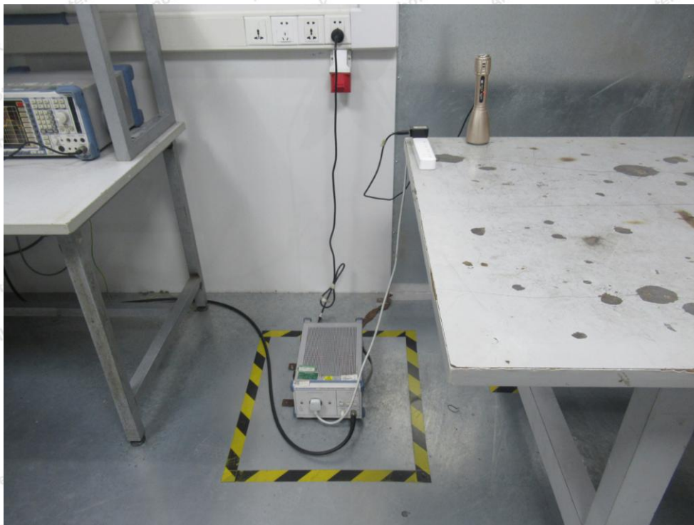
Photo of Conducted Emission Measurement
