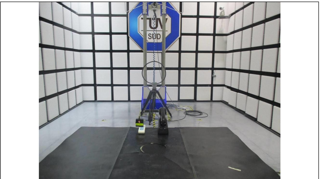
Radiated Emission test (30MHz to 1GHz)
