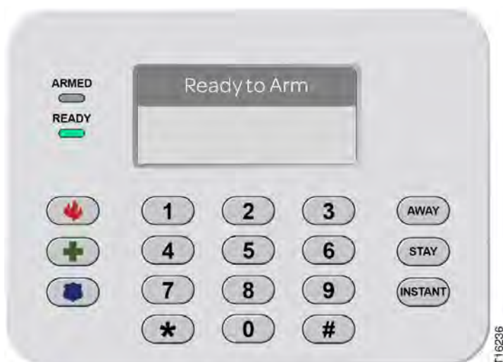
Figure 107: Keypad (Model SR-KPD02)—Ready to Arm
