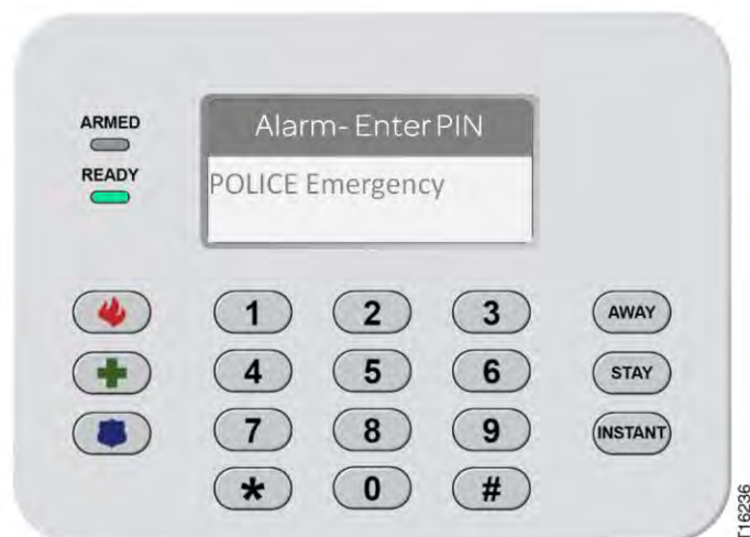
Figure 118: Keypad (Model SR-KPD02)—POLICE (Alarm- Enter PIN)
