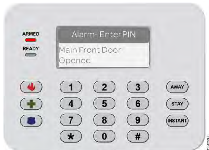
Figure 109: Keypad (Model SR-KPD02)—Alarm- Enter PIN (Triggered Device(s))
