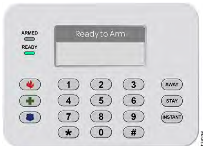
Figure 105: Keypad (Model SR-KPD02)—Ready to Arm
