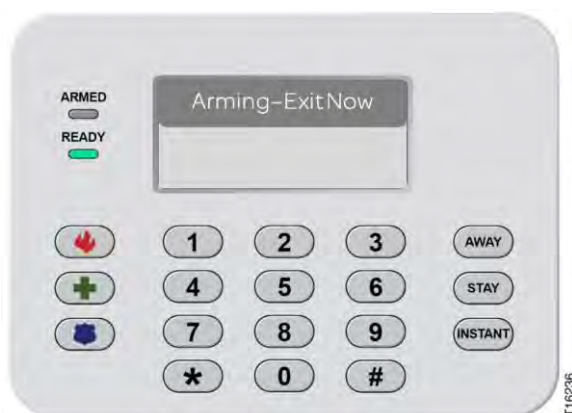
Figure 97: Keypad (Model SR-KPD02)—Arming-Exit Now Mode
