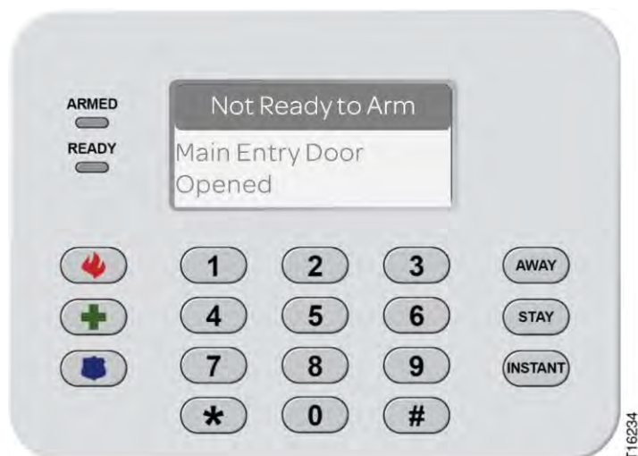
Figure 102: Keypad (Model SR-KPD02)—Open State Device(s)
