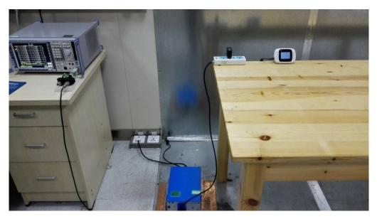
RADIATED EMISSION BELOW 1GHZ TEST SETUP
