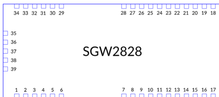
Figure 2. SGW2828 Pin Out (Top View)
