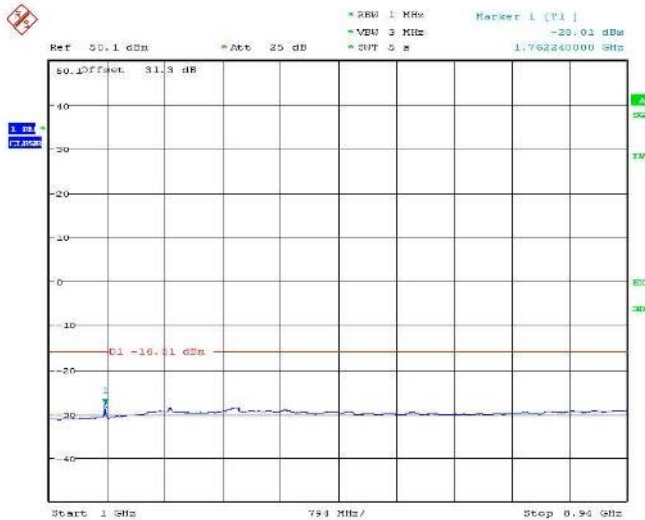
Figure 594 Spurious Emissions (9kHz – 1GHz) - 256QAM (876.5/886.5 MHz) (10+10MHz Channel BW)
