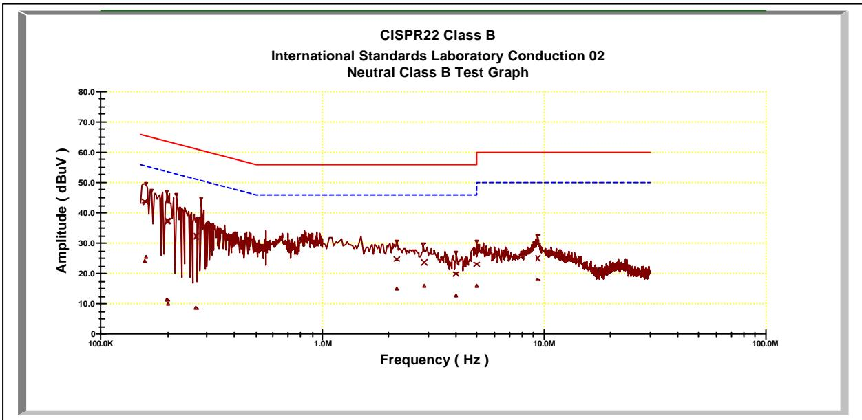
\* NOTE: During the test, the EMI receiver was set to Max. Hold then switch the EUT Channel between 1 , 6, 11 to get the maximum reading of all these channels.
