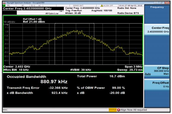
20dB Bandwidth Test Data CH-Mid
