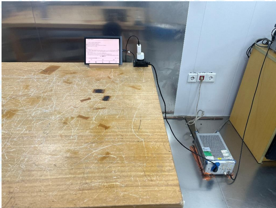
Photo of Setup for Conducted Emission
